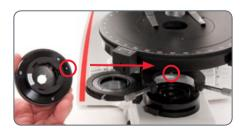
6. Raise the condenser to its highest position using the condenser focus on the left-hand side of the substage
